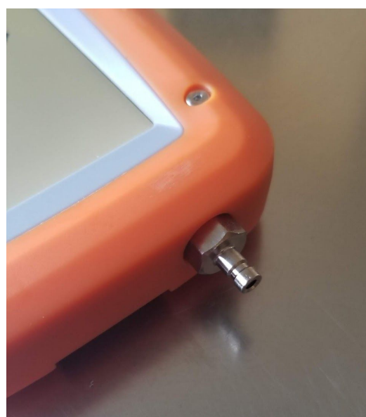
Figure 6: Confined Space Probe attachment point. Always remove probe for storage.
