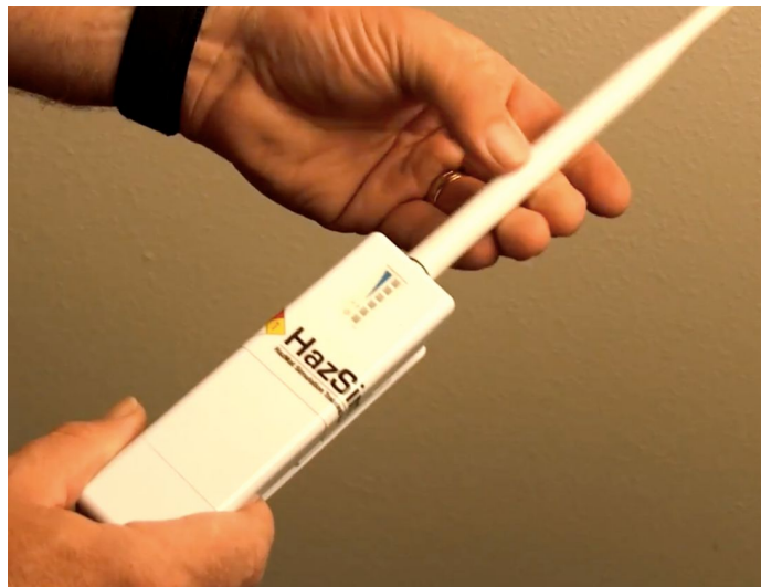
Figure 03: HazSim LAN with screw in antenna. LAN should be placed in a high position for best range results.
